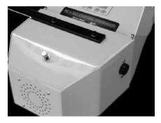
black buttons must be pressed together, to insure that both operators hands are clear of the pressing area, for safety purposes.
